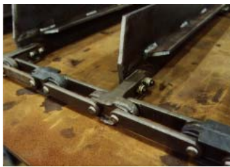
Typical photographs of an assembled chain before and after installation into a scraper conveyor
