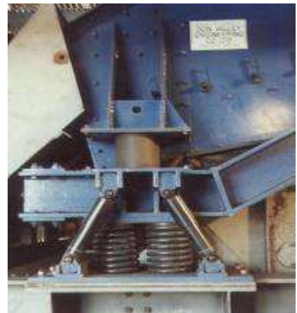
Screen support with anti-vibration Sub frame mounting.
