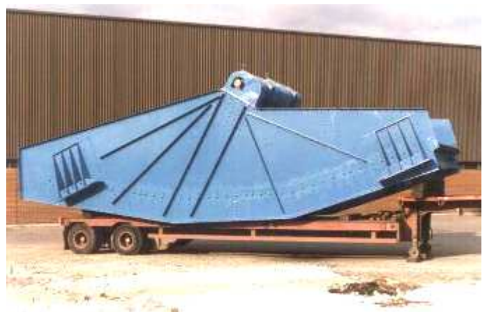
12 meter long multi angle screen awaiting despatch abroad
