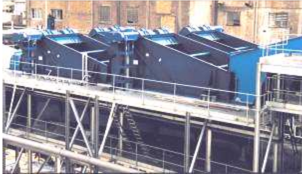
Sugar Beet Dewatering Screens arranged in two parallel lines.
