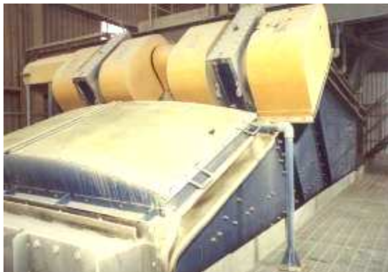
Screen with dust encapsulation
