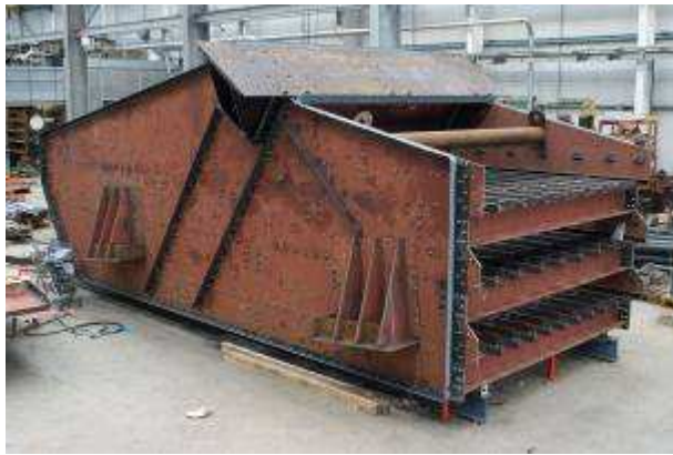
Completed screen carcass
