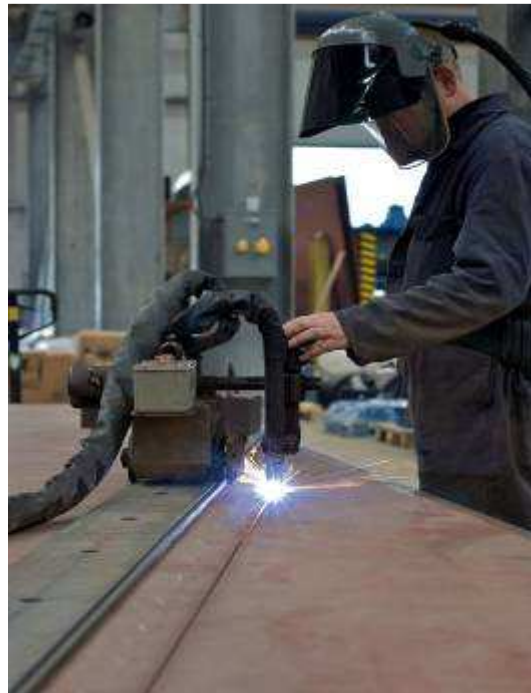
Plasma cutting a side plate
