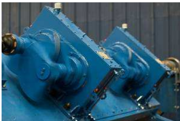
Screen drive mechanisms under pre delivery testing
