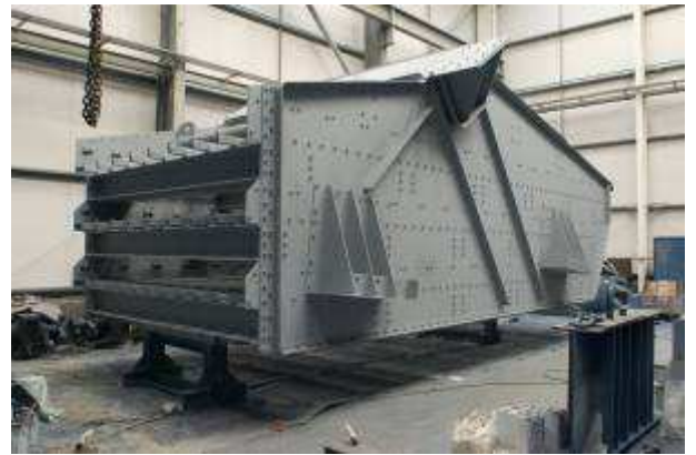
Screen carcass receiving its protective paint finish
