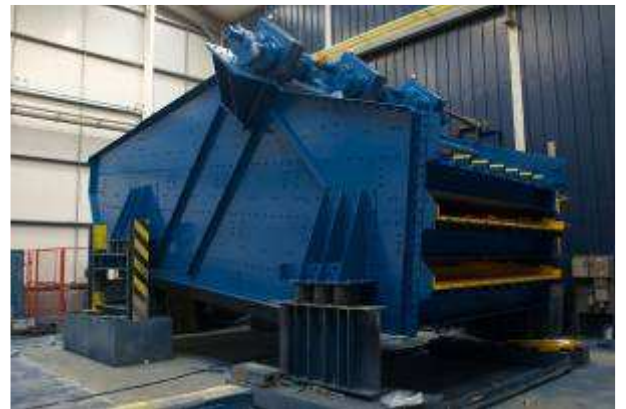
Completed screen under test prior to despatch
