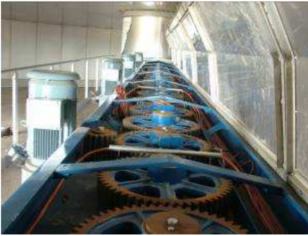
Stripper / loader / turner inside a 30m diameter rotating floor GKV.
