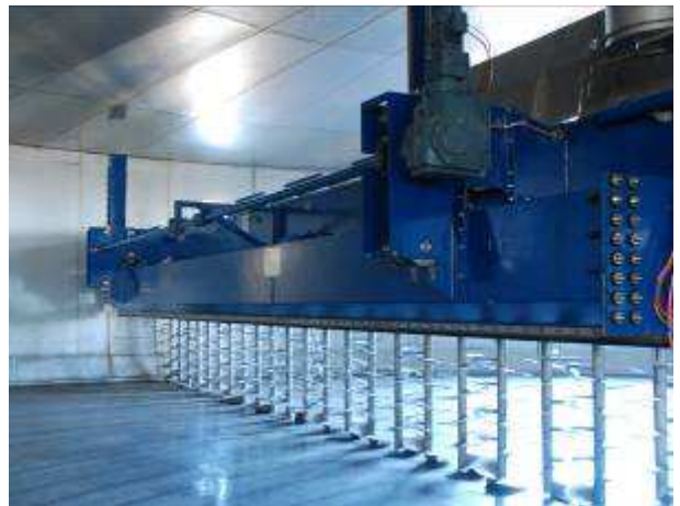
Loader / stripper screw attached to turner beam In its raised loading position.
