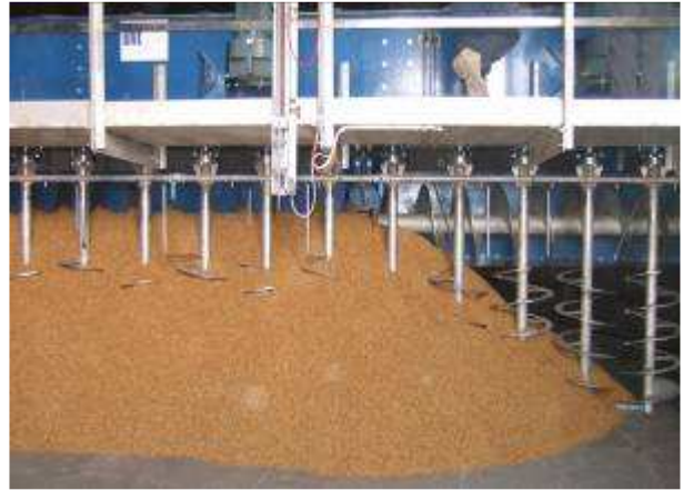
Loading a GKV with distribution screw conveyor in background.
