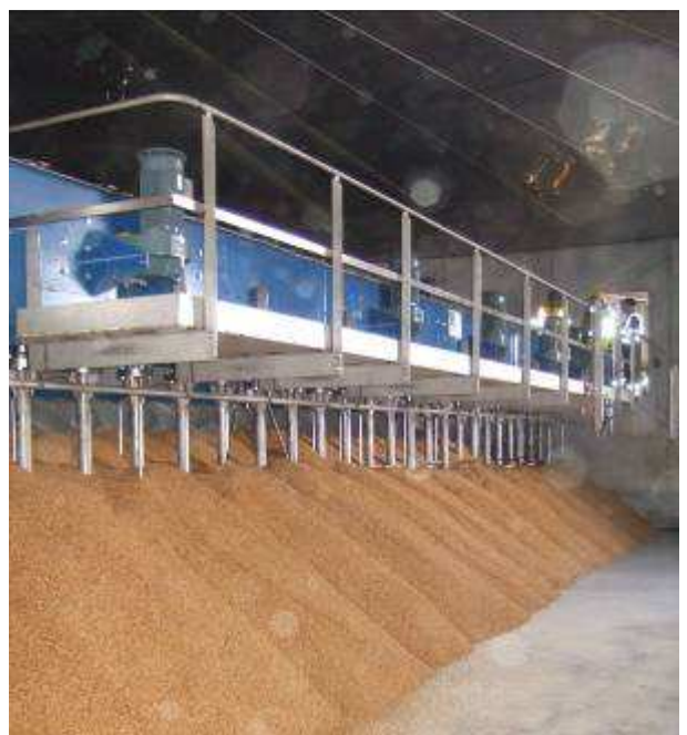
30m dia rotating floor GKV during filling With its 350 te batch.
