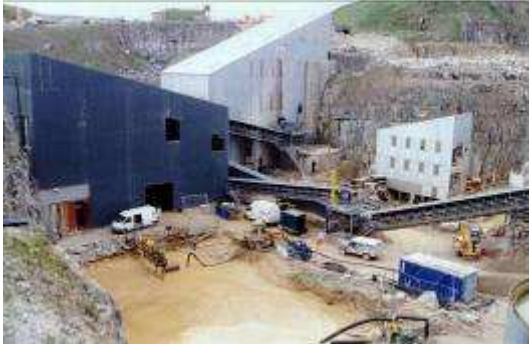
1000 t.p.h. Limestone Washing Plant treating minus 300 mm limestone through twin scrubber barrels.
