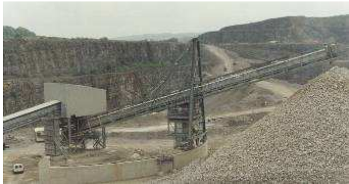
Radial Stacker Delivering up to 2800 t.p.h. minus 254mm Limestone
