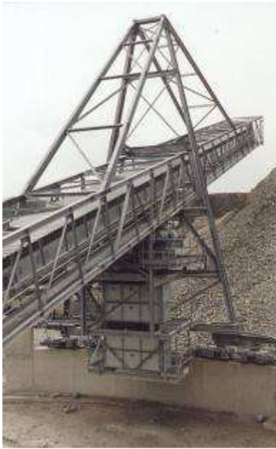
Radial Stacker Delivering up to 2800 t.p.h. minus 254mm Limestone
