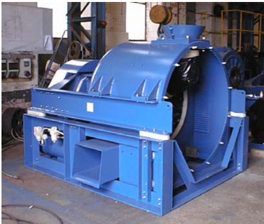
HSG 1100 centrifuge during final stages of refurbishment in our Doncaster workshops.
