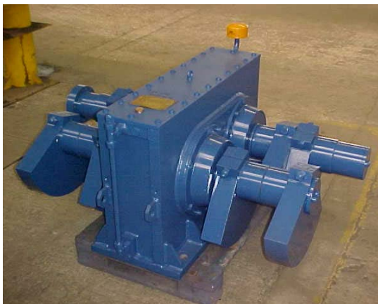
Exciter Unit After Refurbishment
