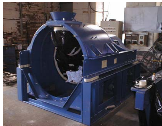
HSG 1100 centrifuge during final stages of refurbishment in our Doncaster workshops.
