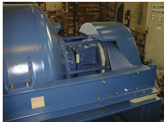
HSG 1100 centrifuge during final stages of refurbishment in our Doncaster workshops.
